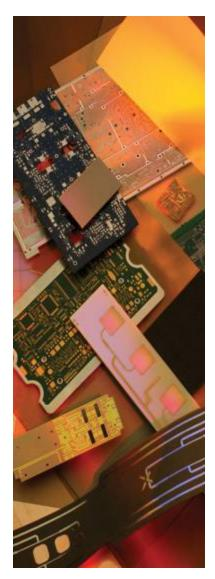
Arlon 92ML ceramic filled thermally conductive multifunctional epoxy laminate and prepreg products are provide best-in-class thermal performance with increased thermal conductivity of 2 W/mK for multilayer PWB's for applications requiring thermal management throughout the entire board volume.
